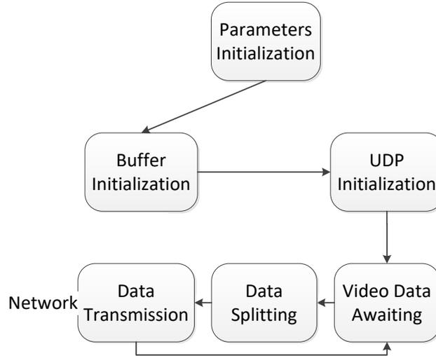
Fig. 5: Working flow for video capture
